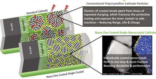
Furthermore, by increasing the ratio of nickel to cobalt in cathode materials, cobalt supply chain risks can be reduced; however, the shift to nickel-rich materials compromises cycle life and safety in the battery. Coated monocrystalline cathode powders can address these problems and the Company's coated nanocrystals provide similar improvements to durability as evidenced through the Company's published results and portfolio of intellectual property.
