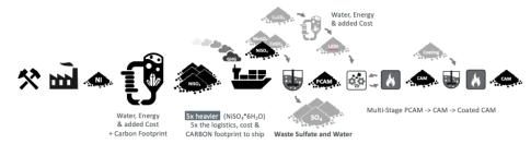
Nano One's patented One-Pot Process forms durable single crystal cathode powders and protective coatings simultaneously and the process has been adapted for M2CAM, enabling these materials to be made directly from nickel, manganese, and cobalt metal powder feedstocks rather than metal sulfates or other salt powders. Metal powders are one-fifth of the weight of metal sulfates, avoiding the added costs, energy, and environmental impact of converting to sulfate and shipping and handling of waste.
